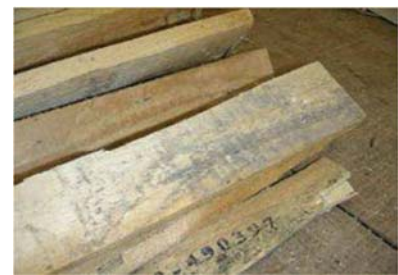
Mold: Not OK
