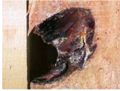
Knot Hole and Resin: OK
