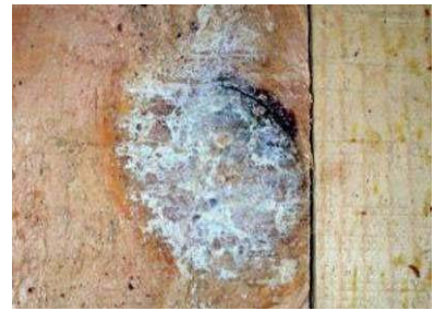
Knot and Mold: Not OK
