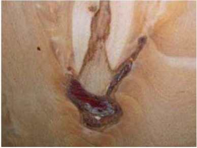
Knot Hole in Plywood: OK
