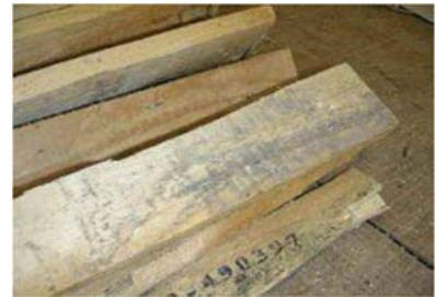
Mold: Not OK
