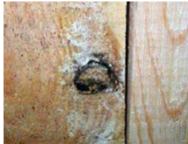
Knot and Mold: Not OK
