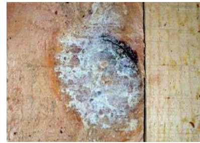
Knot and Mold: Not OK
