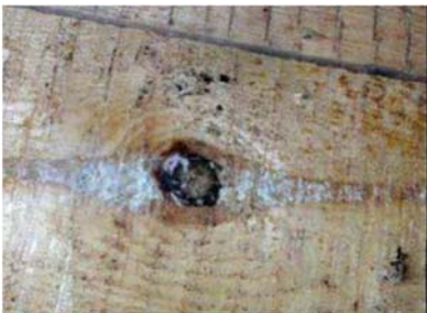
Knot and Mold: Not OK
