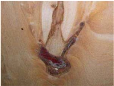
Knot Hole in Plywood: OK
