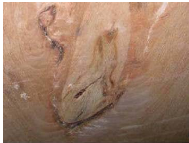
Knot Hole in Plywood: OK
