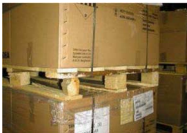
Knot and Mold: Not OK
