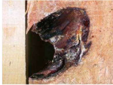
Knot Hole and Resin: OK
