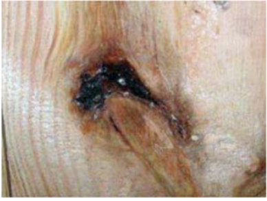
Knot Hole and Resin: OK
