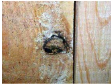
Knot and Mold: Not OK
