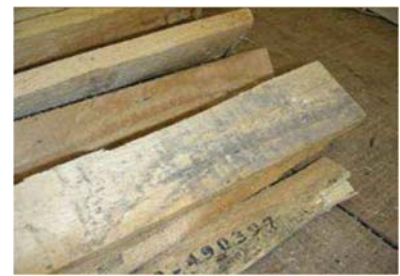
Mold: Not OK
