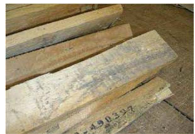
Mold: Not OK
