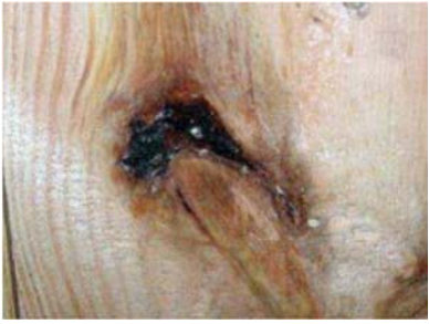
Knot Hole and Resin: OK
