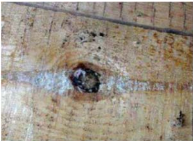
Knot and Mold: Not OK
