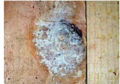
Knot and Mold: Not OK
