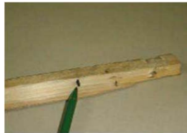
Worm/Pest Hole: Not OK
